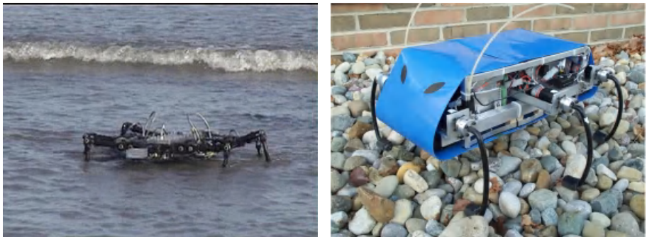
Fig. 2. Biologically inspired robots. Left. Ariel. The first amphibious, legged robot capable of maneuvering in the surf zone. Built by iRobot in collaboration with UC Berkeley. Right. RHex, The robot hexapod capable of negotiating rough terrain using only six degrees of freedom, feed forward control and no external sensing of the environment. Built by University of Michigan and McGill University in collaboration with UC Berkeley.
