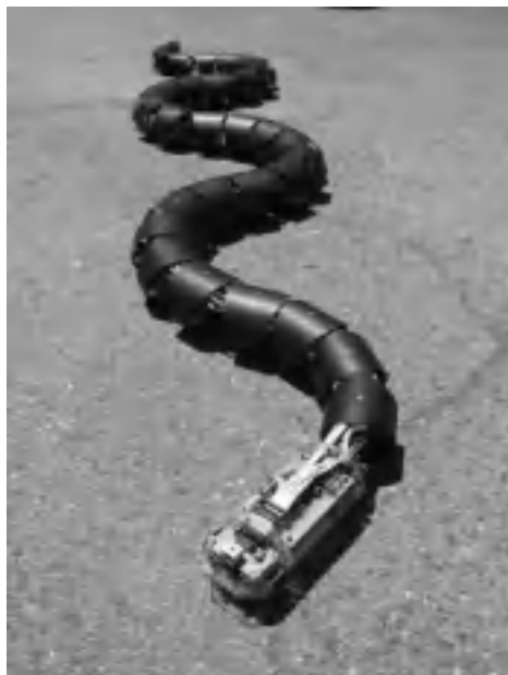
Fig. 1. Gavin Miller’s prototype snake robot S5 performing serpentine locomotion. (Copyright 2000, Dr. Gavin Miller of SnakeRobots.com)
