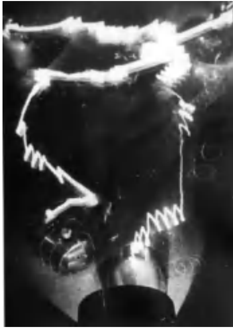
Fig. 7. In this time-exposure photograph, Elmer and Elsie, carrying candles, race for their hutch. Elsie, with the smooth shell, has a bright headlamp that clearly shows the sideways cycloidal movement pattern under low light conditions.
