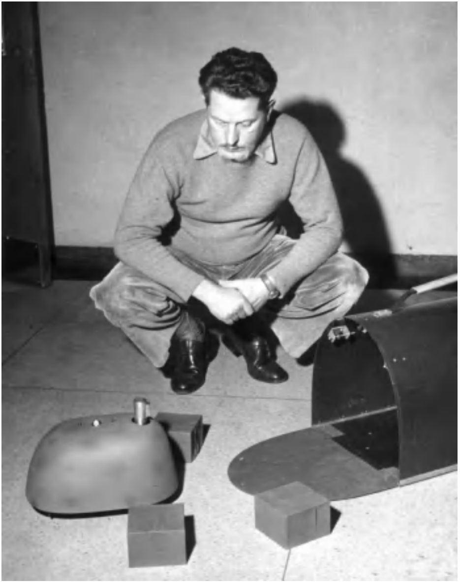
Fig. 13. Grey Walter with a tortoise from the second batch (with an unusual opaque shell) carrying out an experiment on modifying the environment. The boxes are heavy enough to trigger the tortoise's TOUCH behaviour, but light enough to be pushed. (From the Burden Neurological Institute archives)
