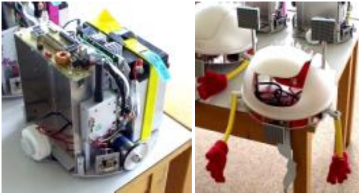
Fig. 16. Robot chassis with body removed and the head and arms of the robot.
