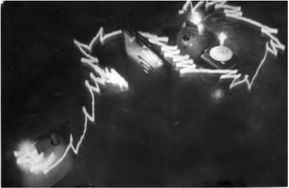
Fig. 9. In this experiment, Elsie encounters an obstacle high enough to obscure the light. She wanders until the light comes into view, and then successfully approaches it.
